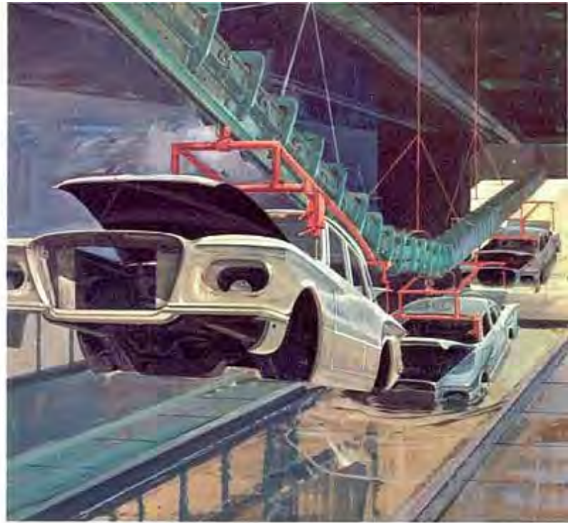
To guard against rust and corrosion the entire lower third of the Valiant unitized body is dipped seven times in cleansing washes and special, protective chemical baths.
